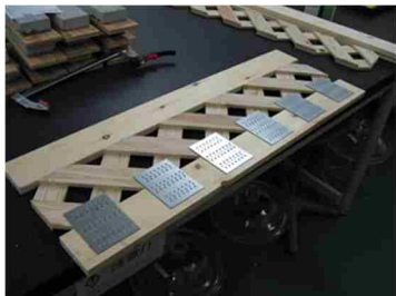
Fig. 5-10 Finish of Nail press
