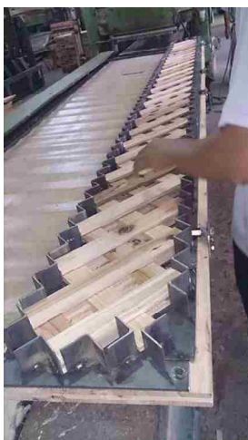
Fig. 2-12 Assembly of lamellas
