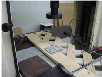
Fig. 5-8 Pressing NP-1 by electric controlled universal testing machine
