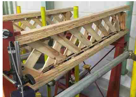
Fig. 4-6 Failure in DOL test of bending
