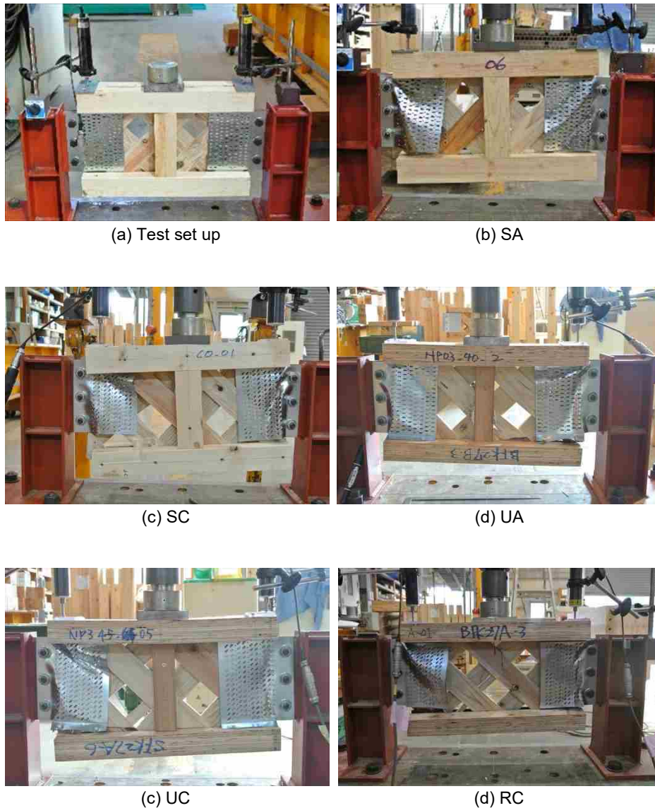
Fig. 5-25 Failure of each type in shear test
