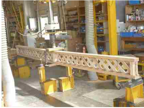
Fig. 3-8 Bending test of 1P-28-41
