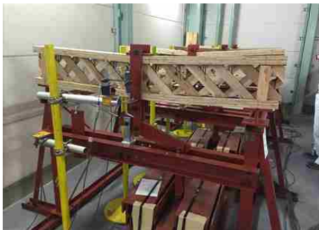
Fig. 4-7 Failure in DOL test of shear
