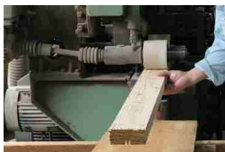
Fig. 2-15 Processing grooves of flanges
