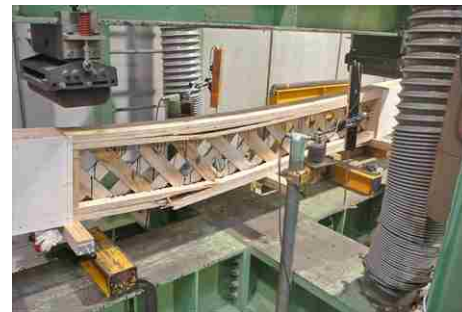
Fig. 3-11 Typical failure in 2P-28-40R
