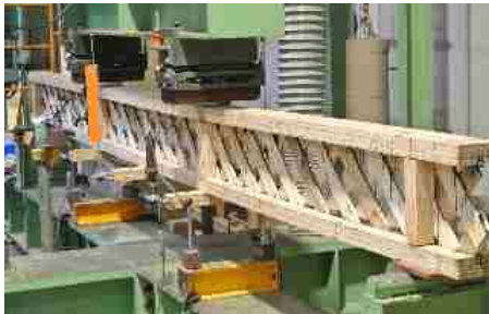
Fig. 3-5 Bending test by two point loading
