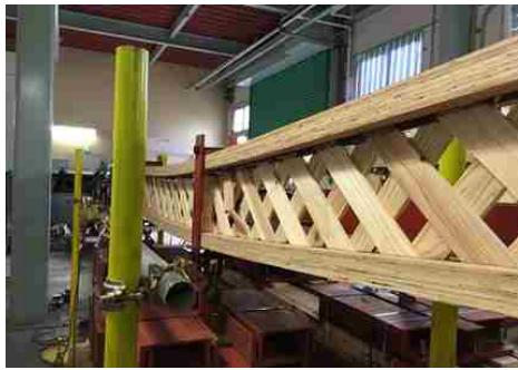
Fig. 4-6 Failure in DOL test of bending
