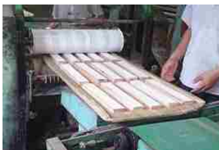
Fig. 2-13 Adhesive application process
