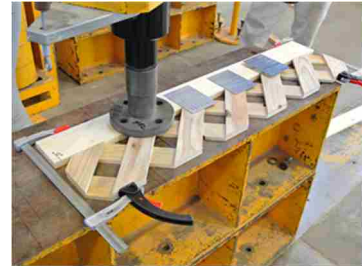
Fig. 5-9 Pressing NP-2 Hydraulic universal testing machine
