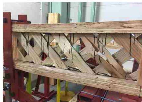
Fig. 4-7 Failure in DOL test of shear
