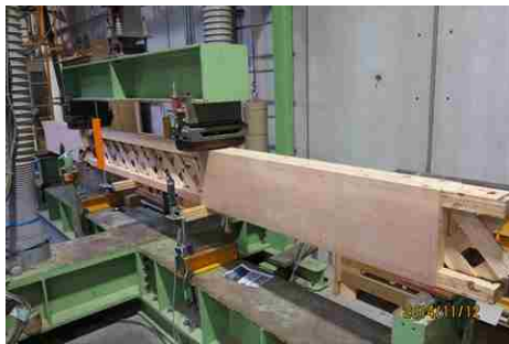
Fig. 3-10 Bending test of 2P-28-40R
