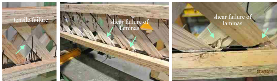
Fig. 3-7 Typical failure in 2P-28-40
