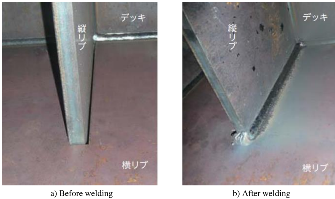
Fig. 4-2 Pictures of the connection between the plate-rib and the non-slit transverse-rib of model PL, before and after welding
