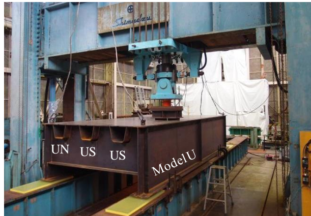
(a) Overview of constant amplitude fatigue test
