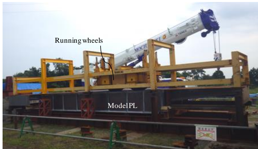
(c) Overview of running wheel fatigue tests
