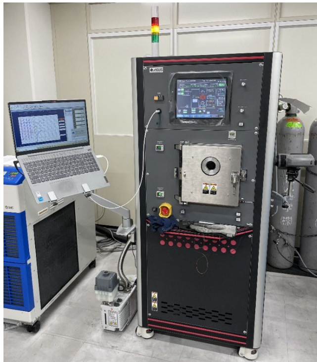
Fig. 2.3 Spark Plasma Sintering.
