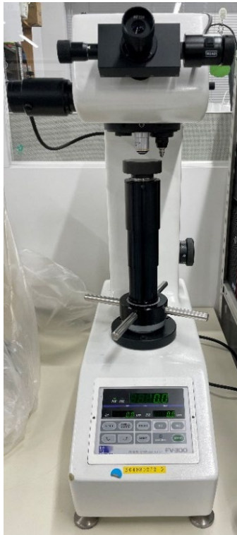
Fig. 2.11 Vickers hardness tester.
