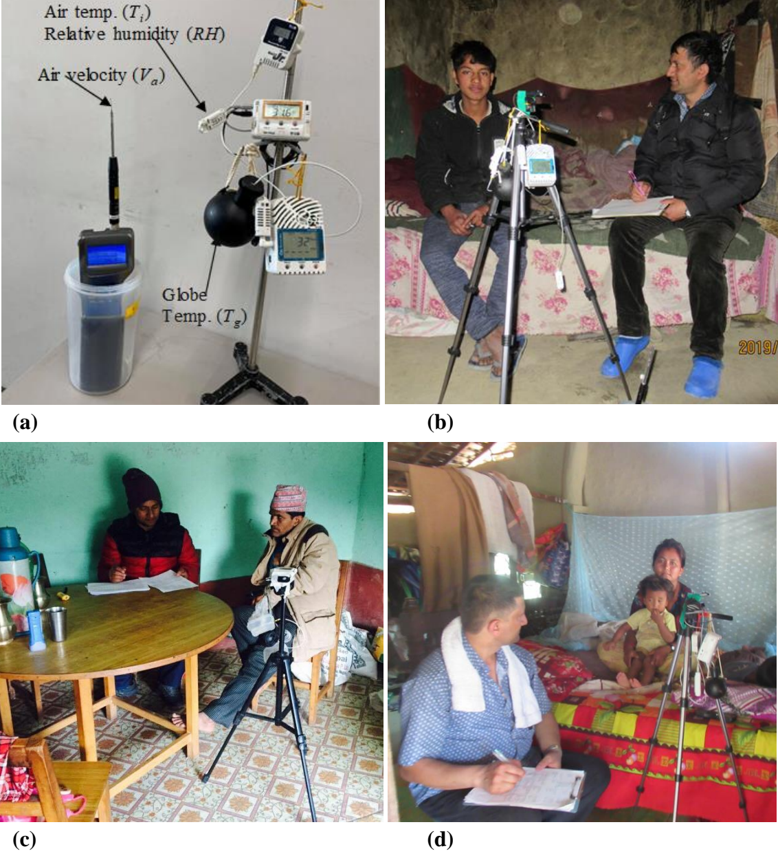
Figure 2.10 Sample snaps of thermal measurement and a scene of interview while performing thermal comfort survey: (a) instruments for thermal measurement; (b) Cold; (c) Temperate, and (d) Sub-tropical regions.
