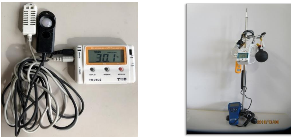
Fig 2.4 Instruments used to measure thermal environmental parameters in study area
